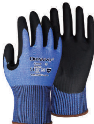
NJ584Q 15G HPPE/glass fiber liner with black micro foam nitrile palm coating, reinforcement at the thumb crotch
